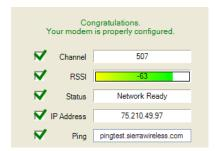
Green checks in the boxes indicate the tests were successful and your RLXIC-ST is functioning properly. At this point your modem is configured and activated to work on your cellular provider network.
