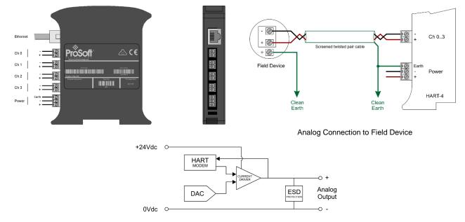
Analog Output Equivalent Circuit
