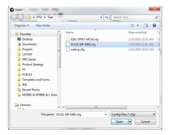
You should now have a PLX31-EIP-MBS configuration in your tree on the left. Right click this PLX31-EIP-MBS and again select Load Config File and click OK to the warning a second time. This time, however, select the WATTCP.cfg that was generated earlier.
