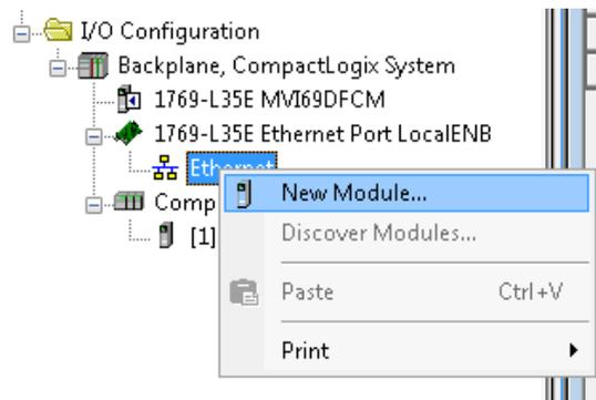
3. In the **Select Module Type** window select a **PLX51-DF1-ENI** module if you already have installed the EDS file if not, you can select a **Generic Ethernet Module**.
