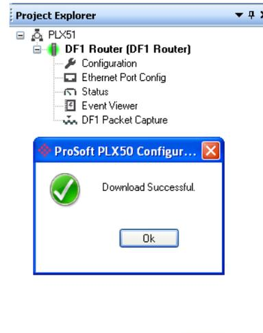
With this configuration the module is ready to route message from Ethernet/IP side to DF1 protocol.
