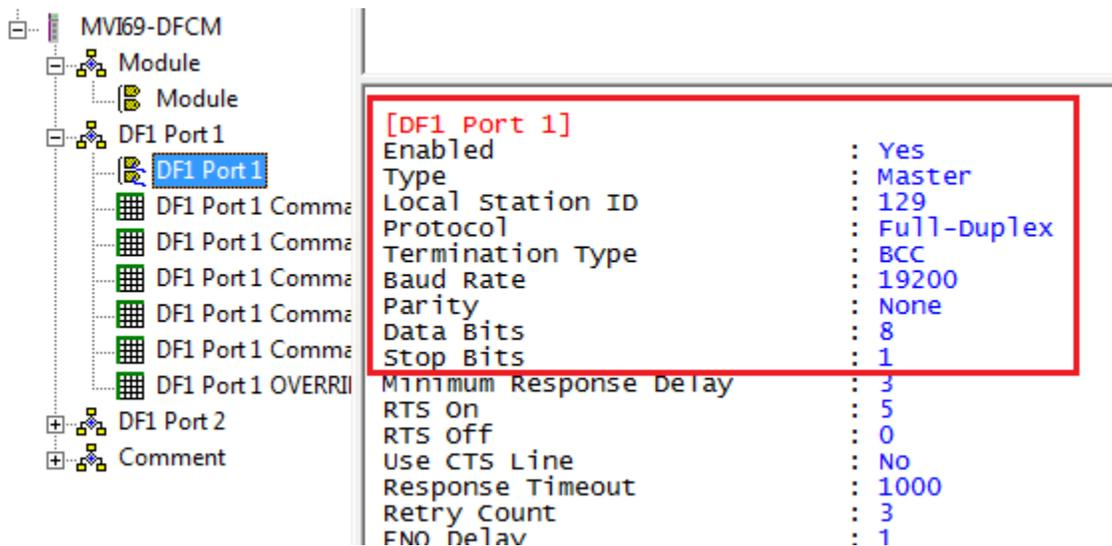
The screenshot shows a tree view on the left with 'MVI69-DFCM' expanded to 'DF1 Port 1'. A configuration window on the right lists parameters for '[DF1 Port 1]'. The parameters are:
