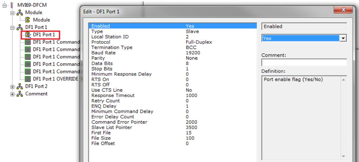
The MVI69-DFCM module is configured under these parameters:
