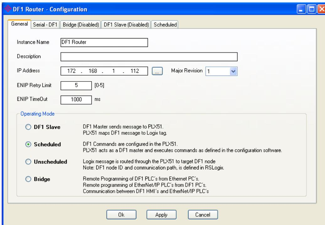
2. In the **Scheduled** tap you need to configure the path to the logix controller using the **Browser** button. Assign a name in **Logix Name** field.
