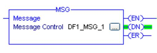
Go to the controller tags then in **DF1\_MSG\_1\_Resp.ResponseData** check if the array has been populated with the values from PLC5.
