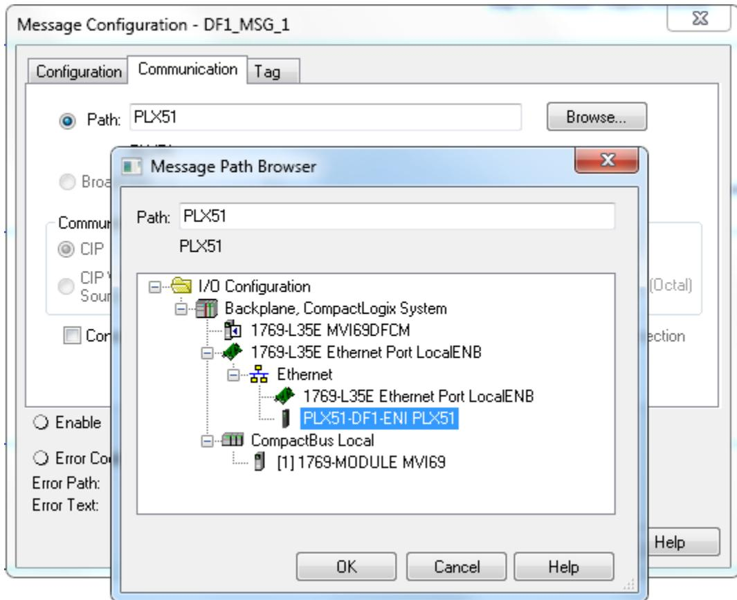
10. Using the tag **DF1\_MSG\_Req** we can configure the command to issue through the Message instruction.
