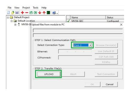
This will upload the configuration from the MVI56-GEC module. Now would be a good time to "Save" the PCB file (or .ppf file).
