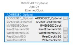
When importing this rung into a program, you may need to change the "Communication Path" of each of the message instructions to match the slot of the module in your program. This can be done by selecting the MSG tag and going to the Communication tab as shown below:
