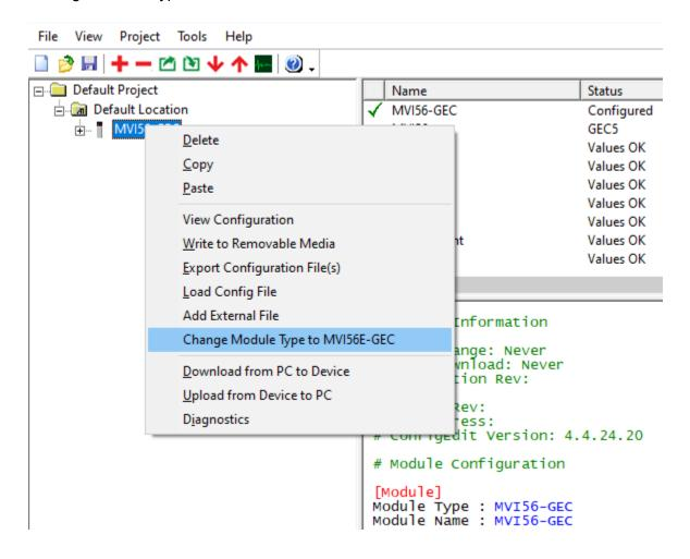
This will automatically convert the configuration file to the MVI56E-GEC.
