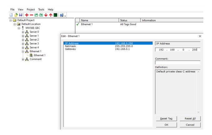
The MVI56E-GEC module uses this IP address for downloading of the configuration file and diagnostics as well as communication with Ethernet devices. The default IP address of the module is the 192.168.0.250 as shown above.
