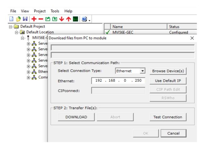
If the module is factory defaults and you are changing the IP address of the module you can select the "Use Default IP" and this will copy the default IP address to the Ethernet settings.
