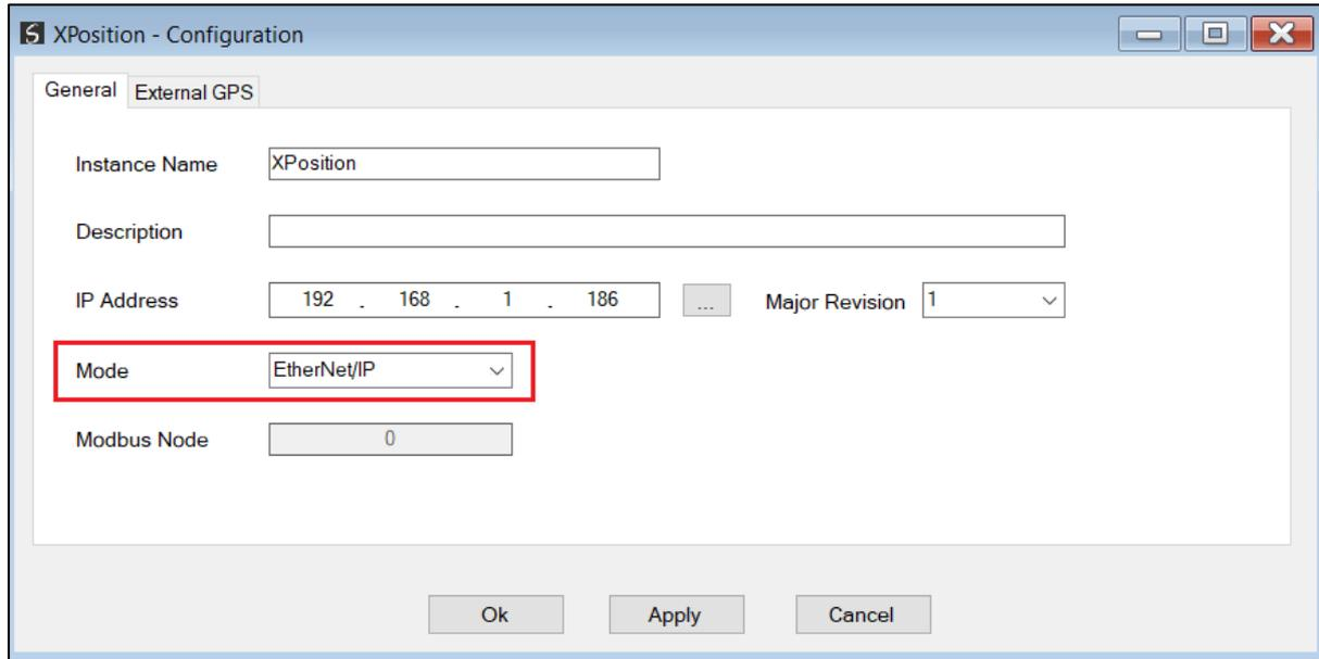
Figure 3.23. – EtherNet/IP mode
