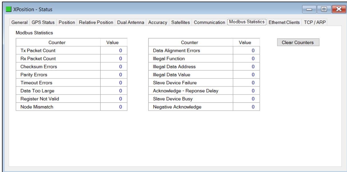
Figure 5.6. - Status monitoring – Modbus Statistics
