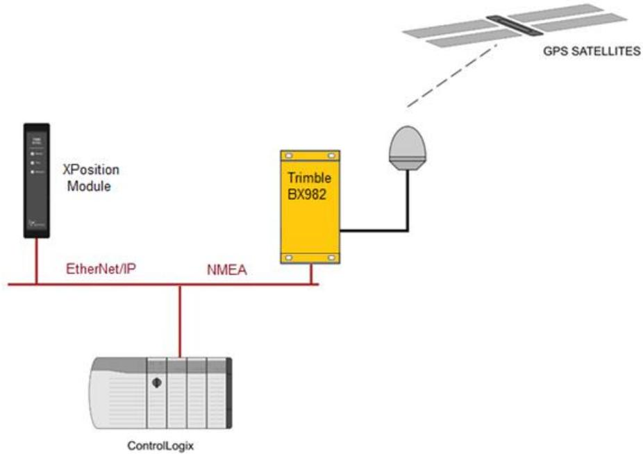
Figure 1.2. - Example of a typical network setup
