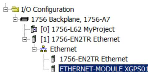
Figure 3.27 – RSLogix 5000 I/O module tree
