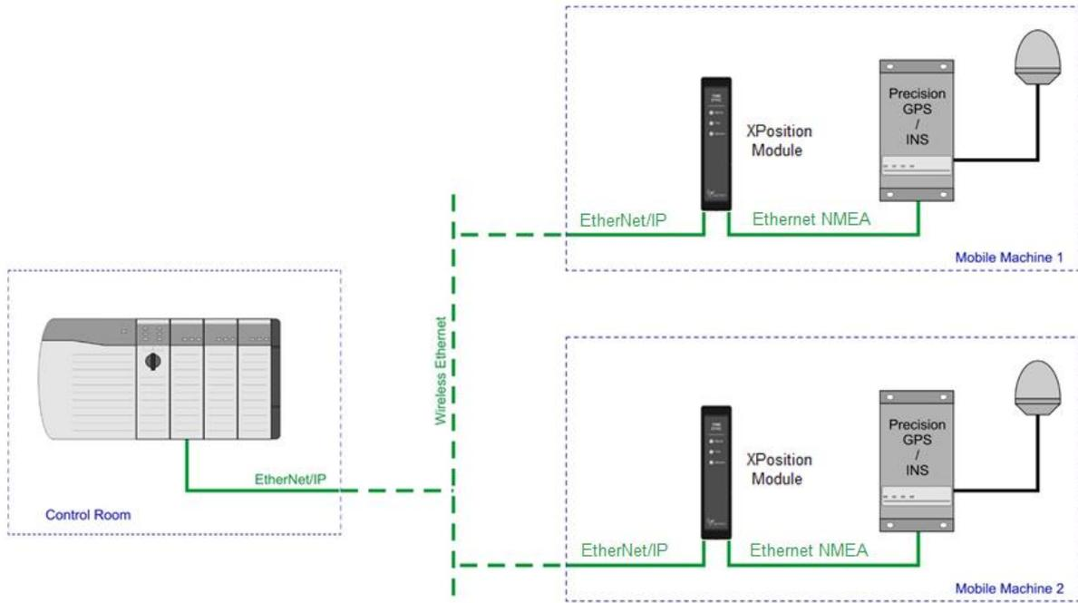
Figure 1.3. - Example of a wireless network setup
