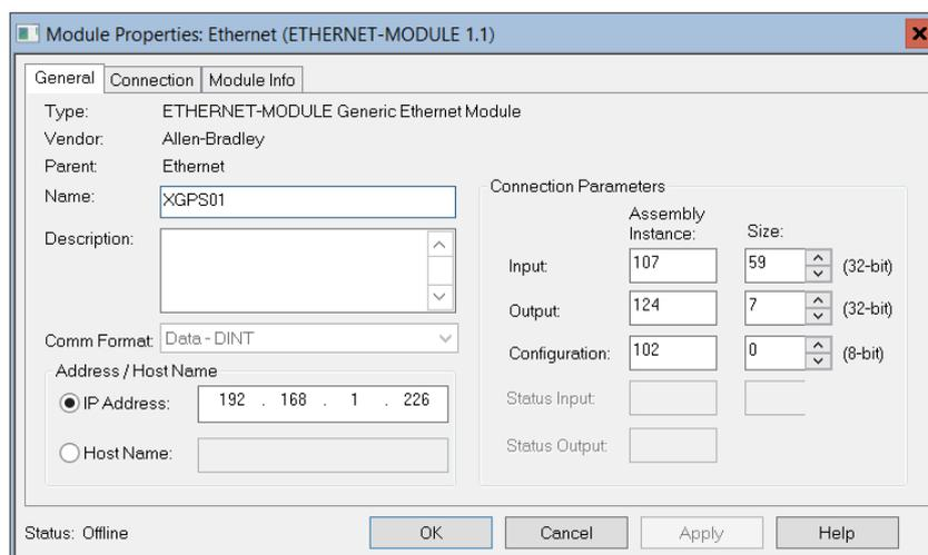
Figure 3.25 - RSLogix General module properties in RSLogix 5000
