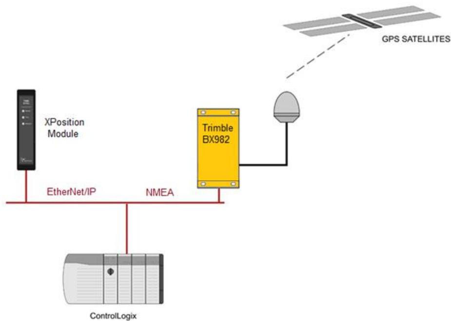
Figure 1.1. – Typical architecture using the Trimble BX982
