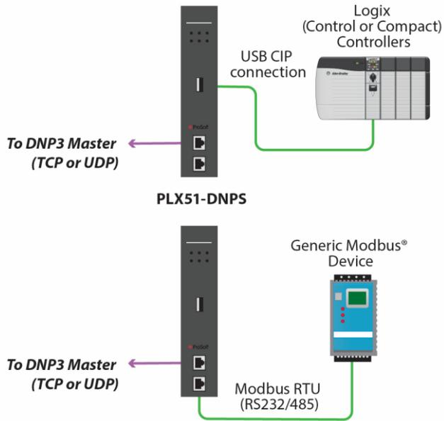
Figure 1 – Flexible connection to Programmable Automation Controllers (PACs)
