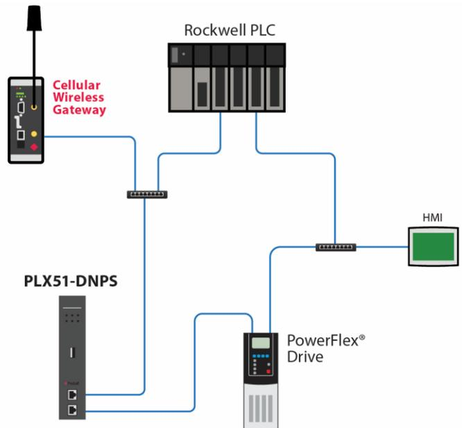
Figure 4 – PLX51-DNPS supports Device Level Ring (DLR)
