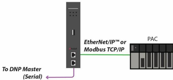
Figure 3 – PLX51-DNPS supports serial or Ethernet connection to DNP3 SCADA Master
