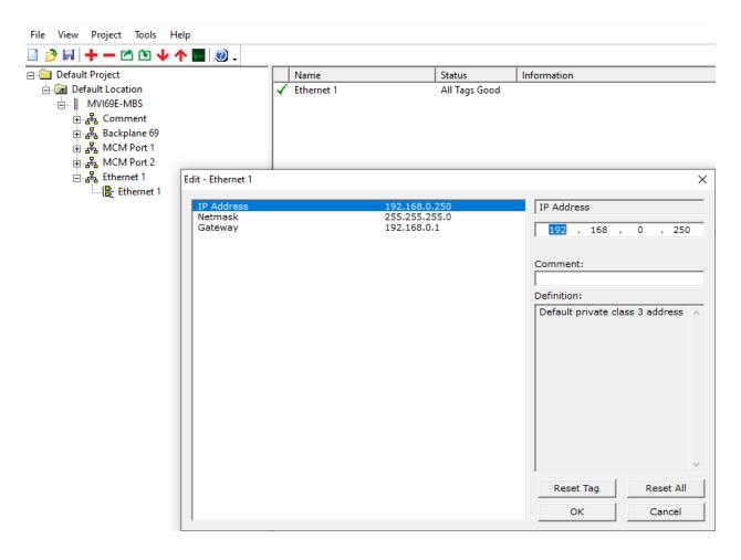
The MVI69E-MBS module uses this IP address for downloading of the configuration file and diagnostics. The default IP address of the module is the 192.168.0.250 as shown above.
