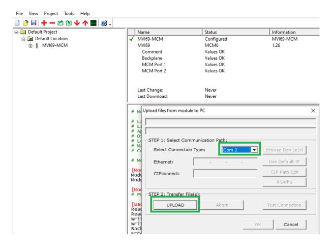
This will upload the configuration from the MVI69-MCM module. Now would be a good time to "Save" the PCB file (or .ppf file).
