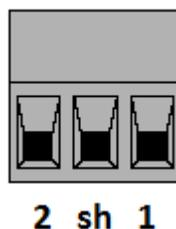
On the AN-X module, the remote I/O connections should be as shown. The wiring in the connector is that same as for the AN-X2 but the connector is rotated 180 degrees on the AN-X4. A remote I/O cable for the AN-X2 can be used without change on the AN-X4.
