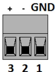
The pins on the power connector are chassis ground, negative voltage and positive voltage. Pin 1 is closest to the Ethernet connector.
