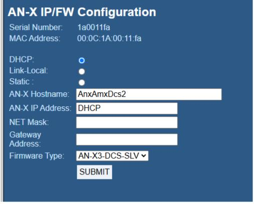
The serial number and MAC address of the AN-X being configured are shown.
