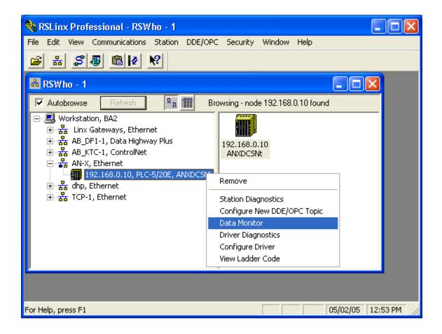
First create an Ethernet driver to communicate with the AN-X3.
