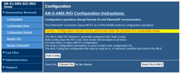
If an Ethernet/IP scanner such as ControlLogix is connected, it must be in PROGRAM mode to use the 'Auto Config' or 'Send File to AN-X' function.
