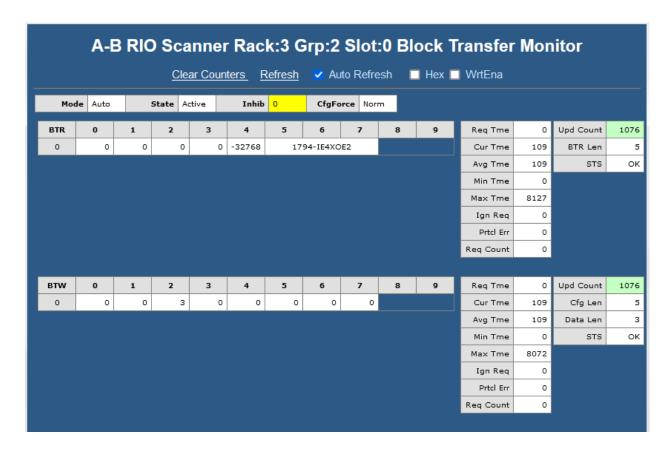
The screen shows the block transfer read and write data for the selected location (rack, I/O group and slot). The last data field shows the first 15 characters of the module name and module type, in this case, 1794-IE4XOE2.
