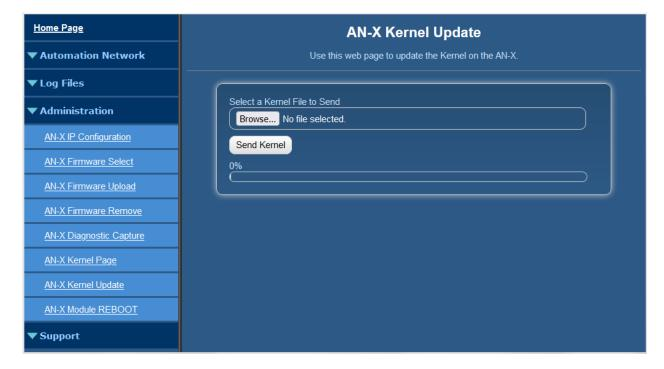
AN-X displays a progress bar as the file is transferred. When the transfer is complete, the AN-X still has to copy the kernel file to the microSD card. When the file copy is complete, the AN-X displays a message to indicate that the file was copied successfully. Stay on this web page until AN-X indicates that the file has been written to the microSD card, then click the REBOOT button to restart the AN-X.
