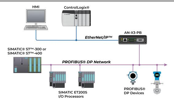
The AN-X3-PB gateway running the HMI firmware acts like a gateway between a PROFIBUS DP network and an Ethernet network supporting EtherNet/IP scheduled connections, PLC5 file emulation, and Modbus TCP.
