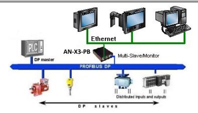
The AN-X3-PB acts as a gateway between a PROFIBUS DP network and an Ethernet network using cyclic UDP messages.
