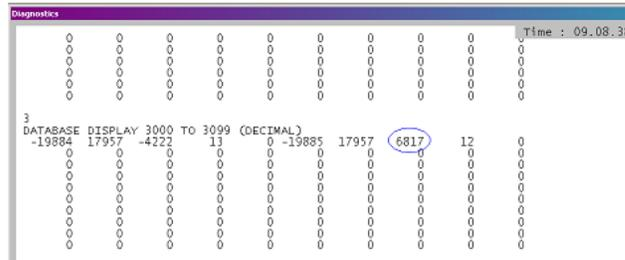
The data shown represents clock values originating from the 6201-WA-DFNT\_150 Client. The values are stored in 10 registers beginning with register 3000. The clock values are being passed wirelessly to the 6201-WA-DFNT Client 151. The 6201-WA-DFNT Client 151 module is taking this data and passing it back to the 6201-WA-DFNT\_150 Client and placing it into 5 registers beginning at register 3005.
