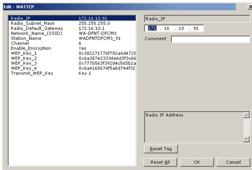
In the sample application, this radio's IP address is set to **172.16.10.91**. In our sample application, the 6202-WA-DFNT-DFCM3 Primary Client IP address is set to 172.16.10.91, so here we used the next IP address in the range which happens to be 90. When you build your own application, you will have to modify the Radio Default Gateway, Network Name (SSID), and Station Name to suit your needs.
