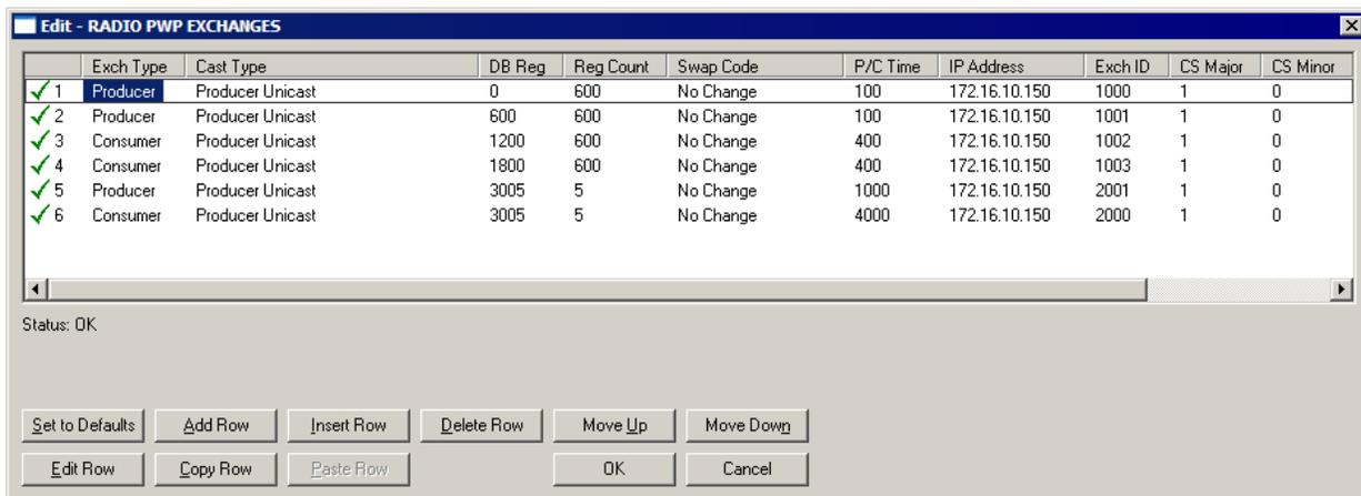
This is the area where you set up data exchange between the DFNT modules. Communication is accomplished using Producer and Consumer commands. Using these commands, you specify the IP address of the receiving (Consumer) and sending (Producer) module as well as the database locations to produce data and receive data.
