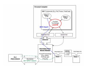
Typical FDT frame applications are Fieldcare (Endress + Hauser), PACTware (PACTware association) or fdtCONTAINER (MM-Software). The PROFIBUS DPV1 master modules support Class 1 and 2 services thereby allowing for PLC cyclic Class 1 services to co-exist with acyclic comDTM Class 2 services over the same network.
