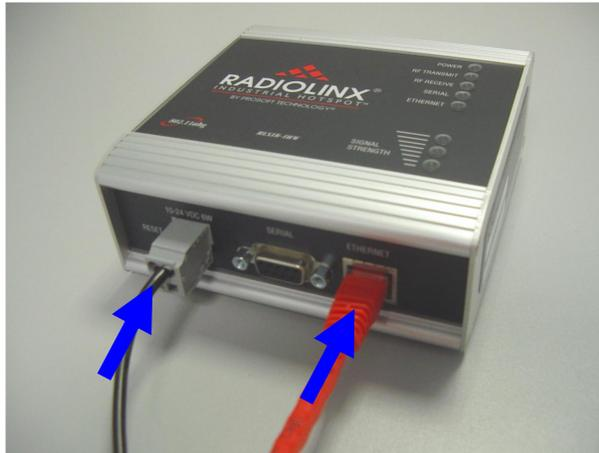
From left to right: Power connector, serial port and Ethernet port.
