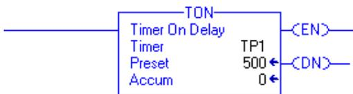
We will use the done bit of the Timer to enable/disable the messages instruction. Into the Rung 0 insert **XIO tp1.DN** as TON condition:
