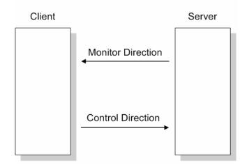
The points that are typically transferred from the server to the client are also known as **Monitor Points** (or Monitor Information Objects). The points that are typically transferred from the client to the server are also known as **Control Points** (or Command Information Objects).
