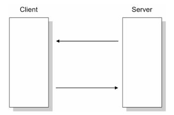
The 4205/5205-TS-104S-PDPS works as an IEC-60870-5-104 server; it can send monitor data, receive commands, or generate events to the client unit.
