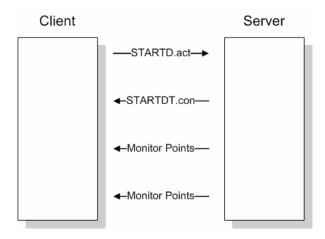
In some circumstances the client unit may not support STARTDT and STOPDT messages. The module may also be tested with simulator software that does not support these features. During these situations, you may want to disable the STARTDT and STOPDT features using the following parameter:
