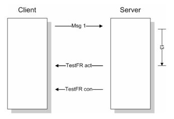
If the module does not receive the TESTFR.con message within a certain amount of time, it will timeout and close the connection. You can configure the timeout period using the following parameter:
