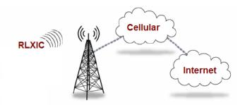
The RLXIC-ST will perform a **one-to-one** routing for all internet traffic to and from the computer or other end device. One-to-one means that your RLXIC-ST will provide a connection for one device to the Internet at a time. In Private Mode, the RLXIC-ST will provide NAT (Network Address Translation) for the computer or other end device.
