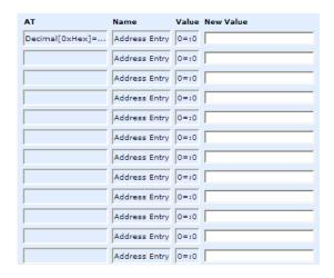
Addresses can be entered in decimal or hex. AceManager will translate hex entries into decimal. The number before the "=" is ID, the number after is the IP address. There can be a total of 100 remote ID/Local addresses entered into the modem.
