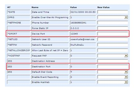
The destination port for the modem at the host needs to match the device port (\*DPORT) in use on all the modems at the remote sites. For example, if the remote modem's device port (\*DPORT) is "12345", then the Modbus host modem's *S53* destination port should be set to "12345".
