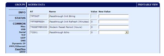
PassThru Mode allows only specific AT commands. Some ALEOS commands will be unavailable when the RLXIC-ST is in PassThru mode. The commands usable also depend heavily on the modem model number (found on the label on the top of the RLXIC-ST).
