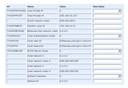
Using a private IP insulates the PPP client from changes in IP addresses of the underlying network. The will perform basic NAT-like address translation on all packets.
