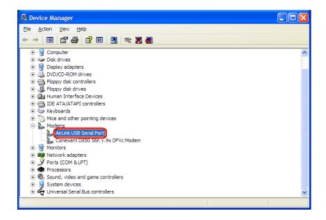
To connect to the modem using the USB virtual serial, most applications or utilities will require you to select or enter the serial (COM) port number. The USB connection will appear as a standard serial port, so you will need to determine its number to connect to it. The driver installation will automatically assign a port or you can change it if you wish to another unused port.
