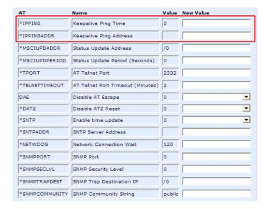
\*IPPING sets the interval, in minutes, you want Keepalive to test the network connection. To disable Keepalive, set \*IPPING to 0 (default setting).
