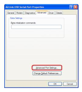
3 At the bottom of the screen, the current port used will be listed. Use the drop down menu to select an available COM port number if you need to change it.
