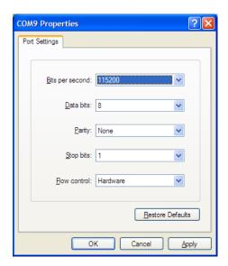
**Tip:** If you have configured the RLXIC-ST for settings different from the defaults for Bits per Second, Data Bits, Parity, and/or Stop Bits, you will need to use your changed settings.
