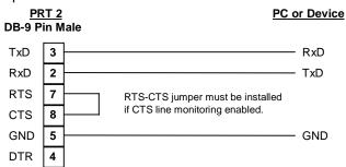
NOTE: If the port is configured with the "Use CTS Line" set to 'Y', then a jumper is required between the RTS and the CTS line on the module connection.
