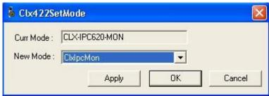
Select the 'ClxIpcMon' mode and hit 'OK' to download the Monitor firmware to the QTS module.
