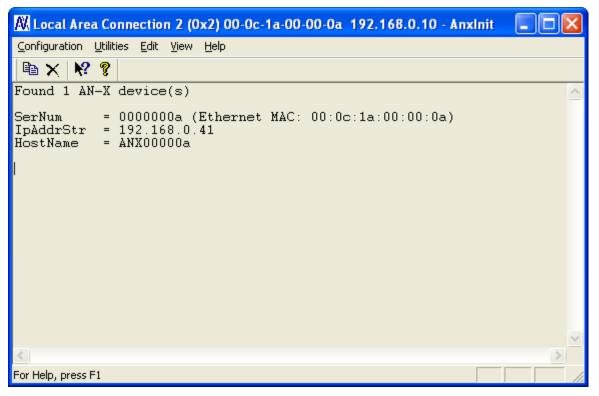
If AN-X does not find a DHCP server within about three minutes of starting up, it reverts to a temporary static IP address of 192.168.0.41 If
