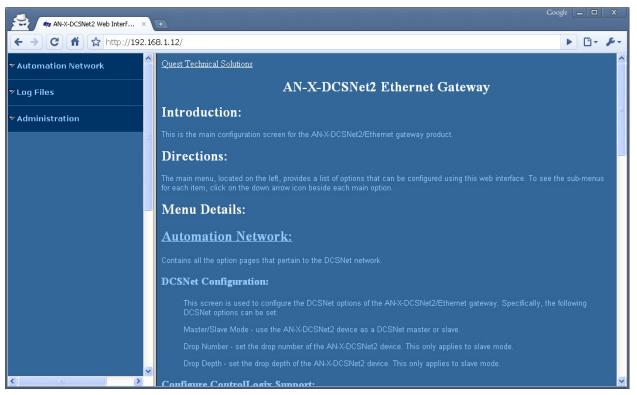
The left pane contains commands. Click on the arrows at the left of the main headings to expand or contract the sections.
