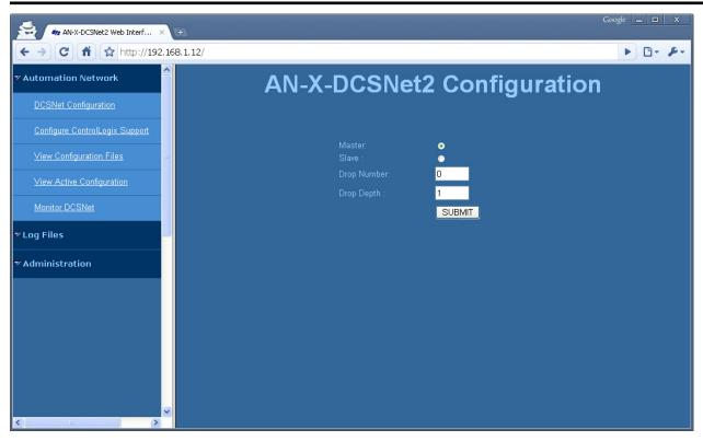
AN-X-DCSNet can be used as a DCS master or slave. Check Master or Slave to select which one you want.
