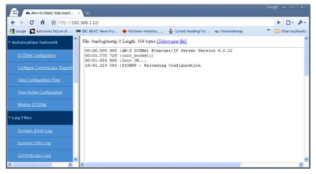
If the log overflows, AN-X closes the log file (enetip.0) and opens a second log file (enetip.1) and continues to alternate between the two log files as each one fills up. Use *View All Logs* to view both log files.
