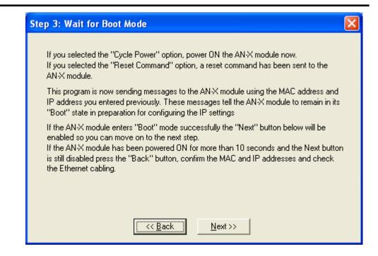
If the AN-X does not enter boot mode within about 10 seconds, return to the previous screens and check the entries.
