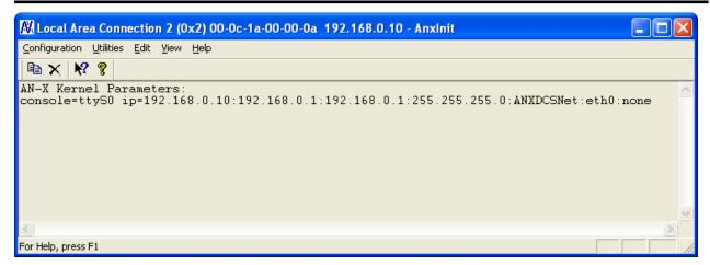
The *Utilities/Read Kernel Parameters* command leaves the AN-X running the boot code. Use the *Utilities/Restart AN-X* command to restart the AN-X in production mode.
