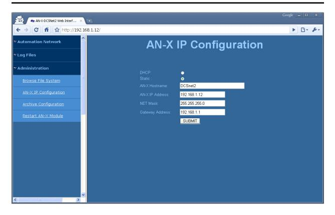
You can configure the AN-X to use DHCP or to use a static IP address.
