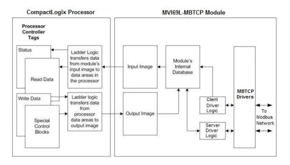
All data transferred between the module and the processor over the backplane is through the input and output images. Ladder logic is needed in the CompactLogix processor to interface the input and output image data with data defined in the Controller Tags. All data used by the module is stored in its internal database. This database is defined as virtual MBTCP data tables with addresses from 0 to 239 each.
