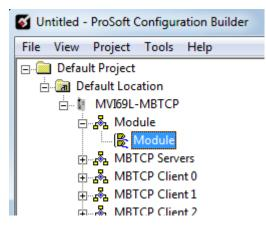
2 Edit the *Slot Number* indicating where the module will be placed in the 1769 bus. The *Slot Number* parameter in the PCB configuration affects the format of the .L5X file that is exported. This parameter identifies the residing slot of the module in the CompactLogix rack.
