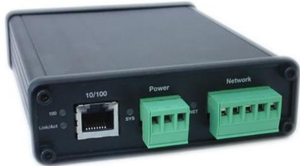
The AN-X2-SQD-MAS communications module connects to a ControlLogix PLC over Ethernet/IP and acts as a scanner on the Square D remote I/O network. It connects to CRM-220/222 adapter modules, NOT Passport I/O.
