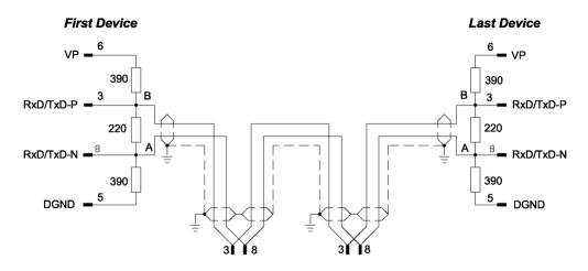
Up to 32 PROFIBUS devices can be connected to one bus segment, without repeaters. If several bus segments are linked to each other with repeaters, there can be up to 127 devices on the network.
